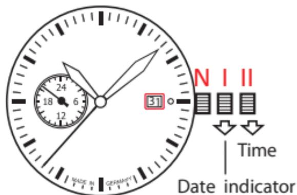
**Date adjustment:** Pull out the crown till position 1 and adjust the date by turning it counter-clockwise, then push the crown back into its neutral position [N].
