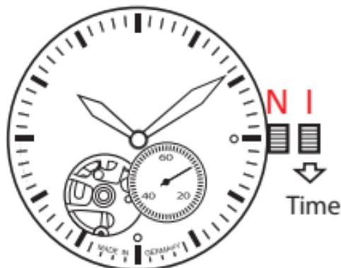
**Time adjustment:** Pull out the crown at position 1 and adjust the time by turning it counter-clockwise, then push the crown back into its neutral position [N].
